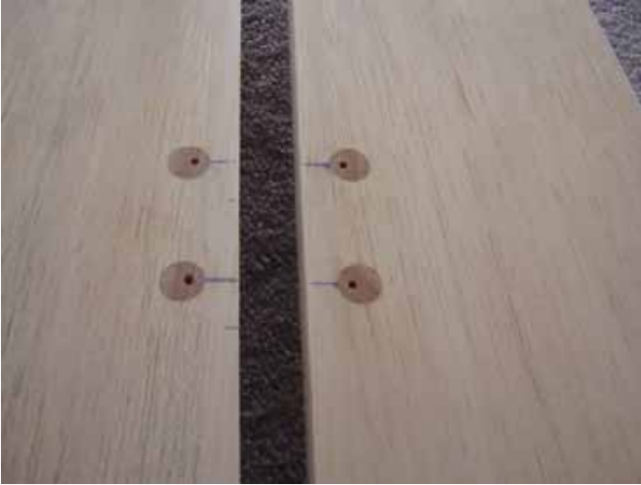
(28) Using 2 t pins locate the center lines on the stabs and elevators.
