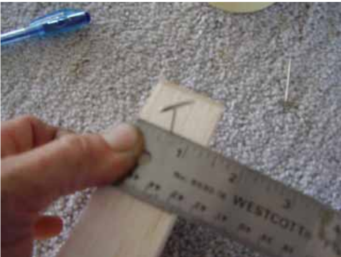
(28) Using 2 t pins locate the center lines on the stabs and elevators.
